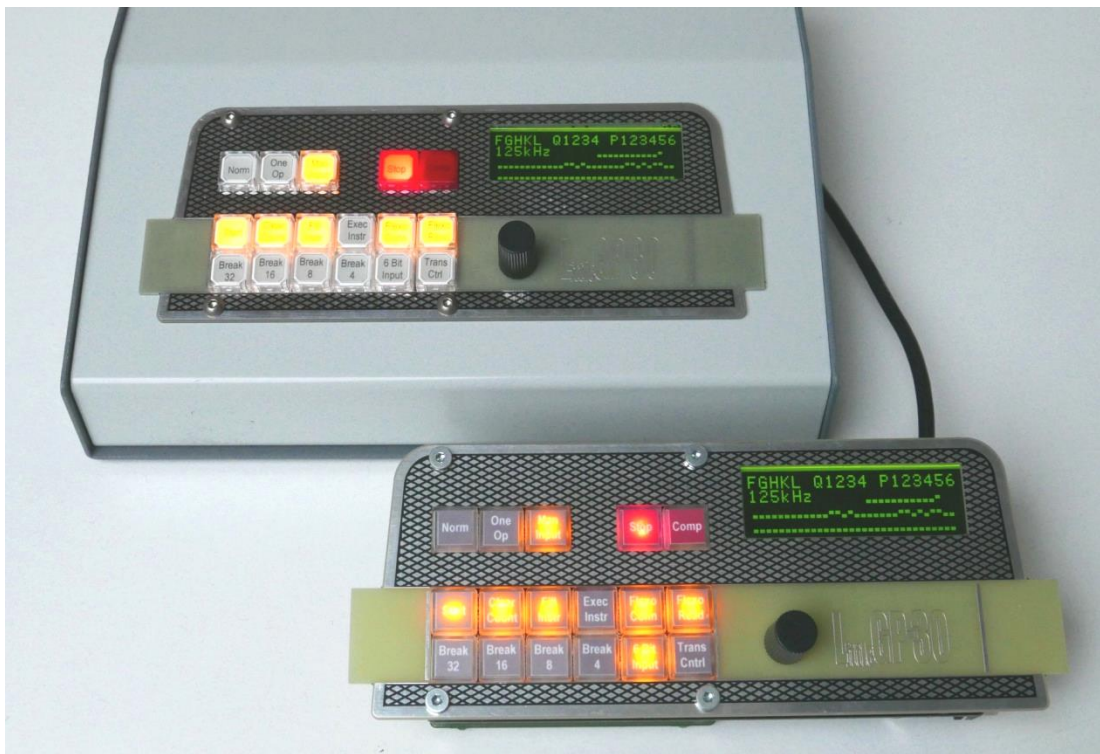
LittleGP-30 with enclosure (Hammond 515-0930) and OMRON switches, and as a bare-board version with Diptronics switches.
