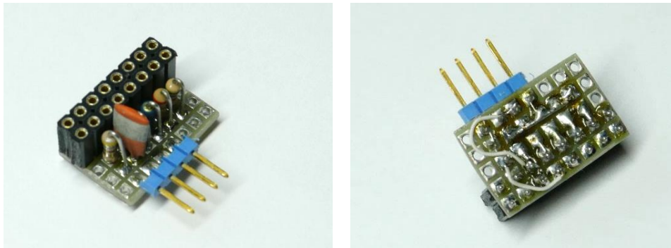
Oscilloscope adapter, hand-wired on perfboard
