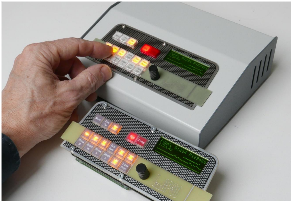
Two ways to build your LittleGP-30: Enclosed (Hammond 515-0930 enclosure shown here) or bare boards.
